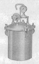
Complete with safety valve, pressure gauge and PT5 heavy duty 3-way air regulator. May be used with any compressed air line. Eliminates need of refilling spray gun cup, since cup is not used. Head is connected to tank with a 15 foot 3% inch material hose and 15 feet 1/4 inch air hose.
